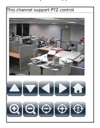
2. You can tap the direction buttons and the zoom buttons to control the camera. Tap the home button to return to home position. You can also adjust the focus of the camera using the focus buttons or tap the autofocus button.
