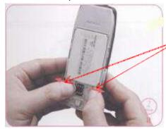
The two clips either side of the SIM section have arrows pointing outwards, push them both out and the battery with pop up.
