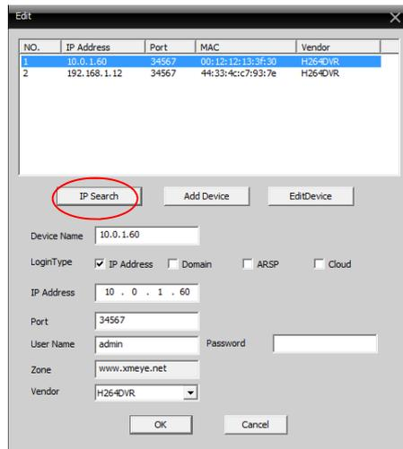
5. Select a camera you want to connect and check that the network setting is correct.
